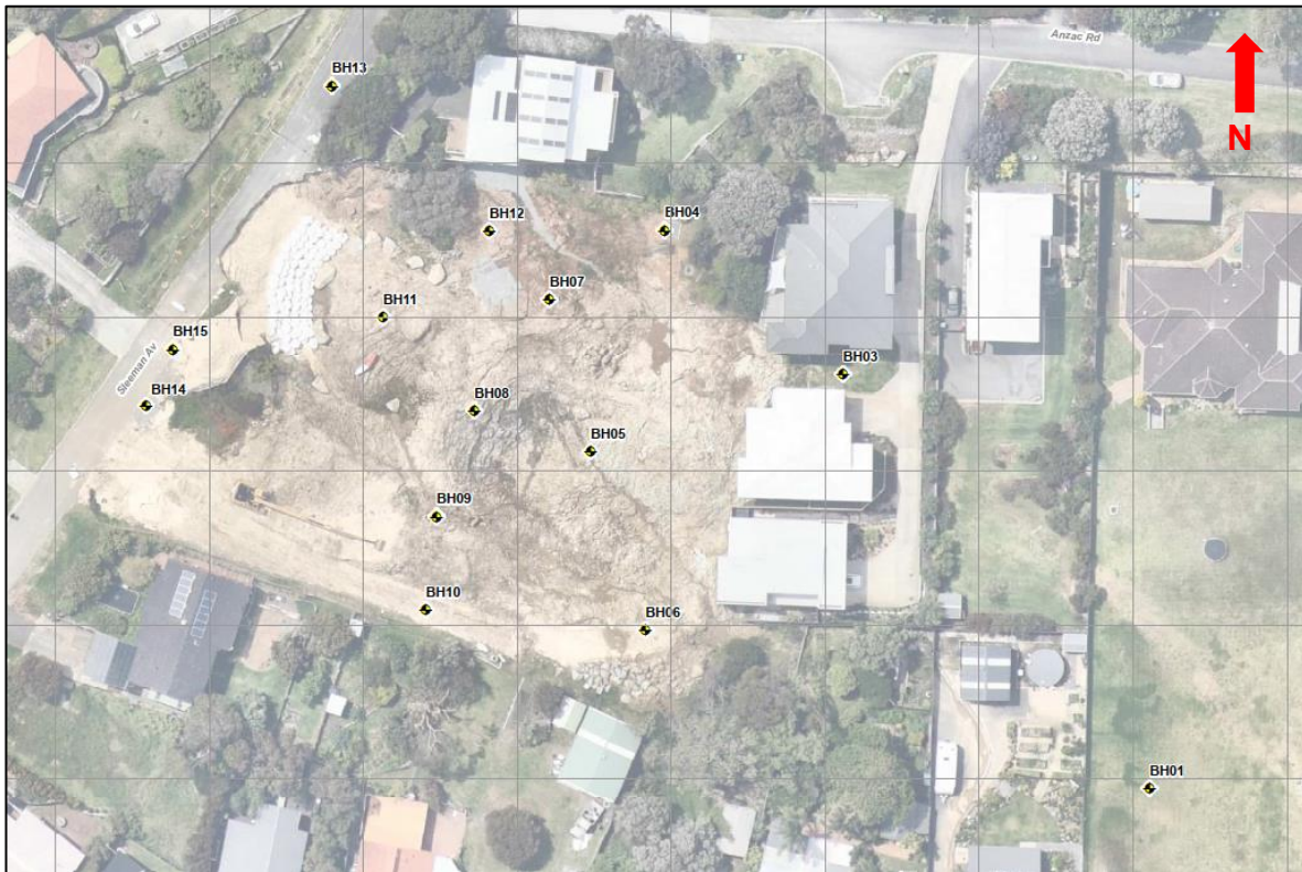
Plate 1: Borehole location plan, CMW investigation December 2022
