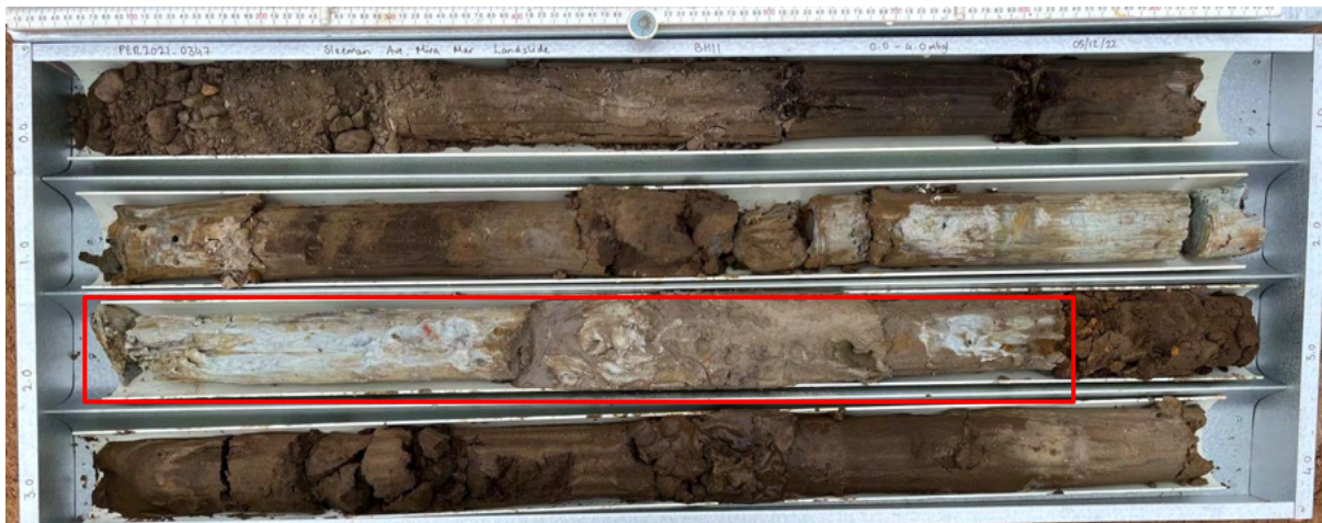
Plate 3: BH11, saturated sand lenses present within the colluvial material.
